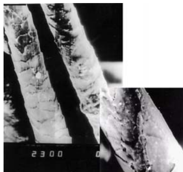
Fig. 16. SEM images of plasma treated wool strand.
